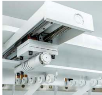
HIWIN ball screw &amp; linear guide
